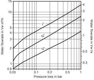
Pressure loss diagram with open valve at 20 °C. The values indicated are applicable to spring loaded valves with horizontal flow. With vertical flow, insignificant deviations occur only within the range of partial opening.
