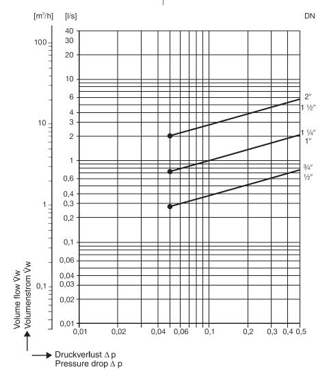
Required minimum volume flow V<sub>w</sub> for equipment with standard spring and horizontal flow.
