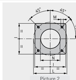
Flange dimensions and boiler drilling template.
